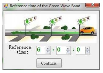
6. Type into the Green wave Refence time ,and press "**confirm**" button . It will give a report about the Green wave menu and solution setting guide.
