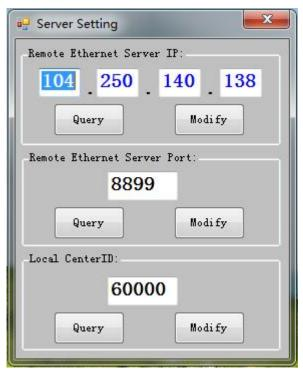
Figure 4 Remote Server Connection Parameters Setting Form
