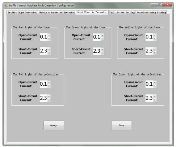
Figure 23. Light Electric Parameter Setting form
