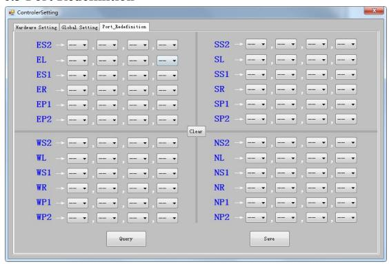
This function is advanced function, you can use at least one output board to control a crossing. Users can freely choose the number of output boards, can freely redefinition the port to what you want to be.
