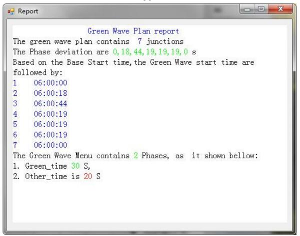
7. According to the data above to plan the green menu and solution in the traffic setting and configure each intersection of the Green Wave band members.
