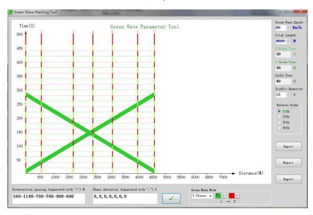
3. Adjust the Green Wave speed to ensure that the Green Wave band line is meet to the green line at the end of the time.
