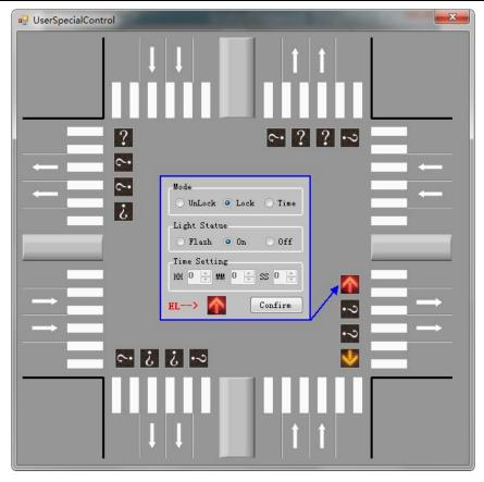
When the command center find clogged intersection, by using the current function, guide traffic to the smooth running of the line, avoid further road congestion.
