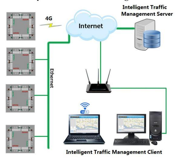
Figure 1. The system architecture diagram
