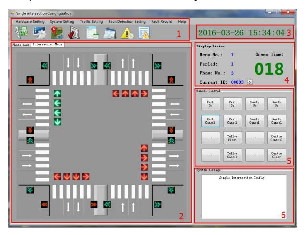
Figure 6 Single Intersection Configuration (Intersection Mode)
