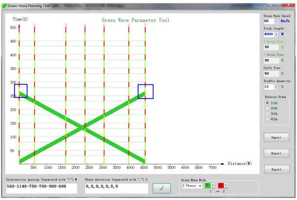
4. Adjust the Phase deviation and press the " $\checkmark$ " to ensure the green line of the each intersection's menu to meet with the Green wave band, as it shown below in blue box.
