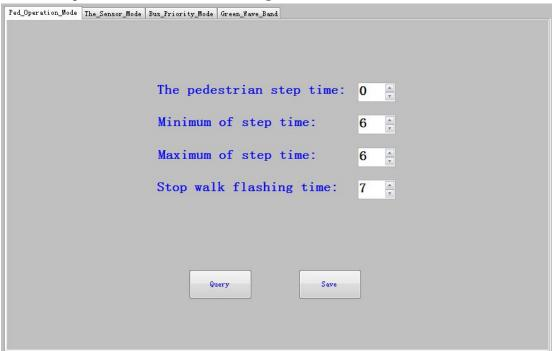
Figure 20. Ped Operation Mode Parameter Configuration form
