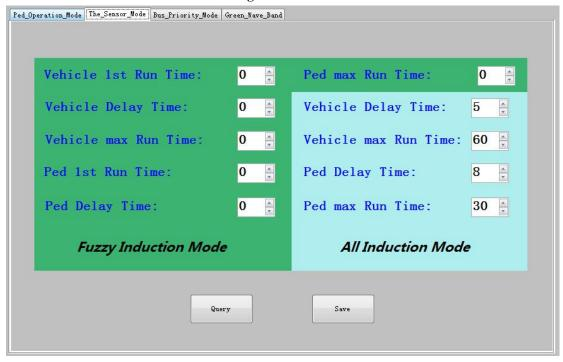
Figure 20. The sensor Mode Parameter Configuration form
